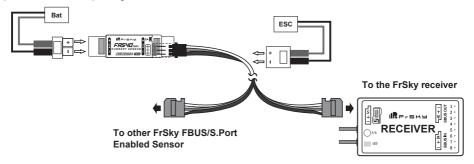
Warning: Install FrSky Current Sensor – FAS40 ADV on any appropriate surface of the airframe that stays away from water, vibration, or fuel.
